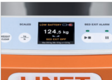
Scales measure with the precision of 0.5 kg
