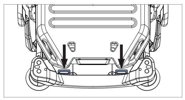
Fig. Two optional holders of the Paper Roll Holder
