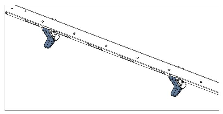
Fig. Positions of both Siderail Release Levers when the siderail is locked
