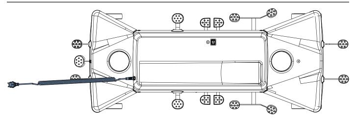
Fig. Power Supply Cord on the head end of the Sprint 200 with scales or with i-Drive Power
