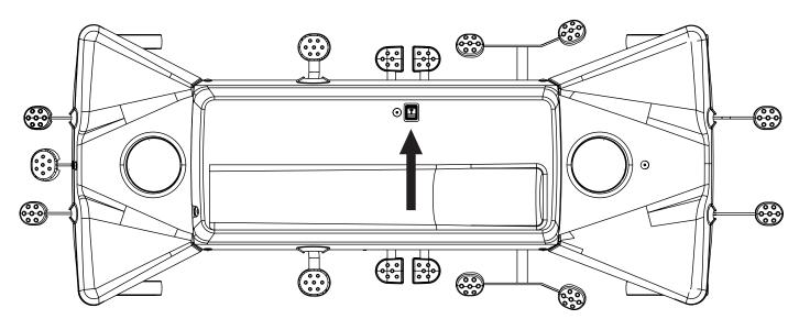
Fig. Position of the i-Drive Power Mains Switch
