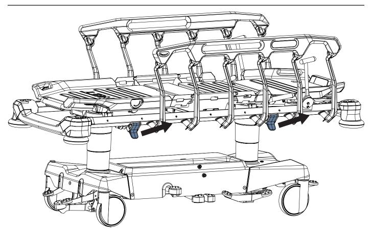
Fig. Release of the siderail at head end and foot end
