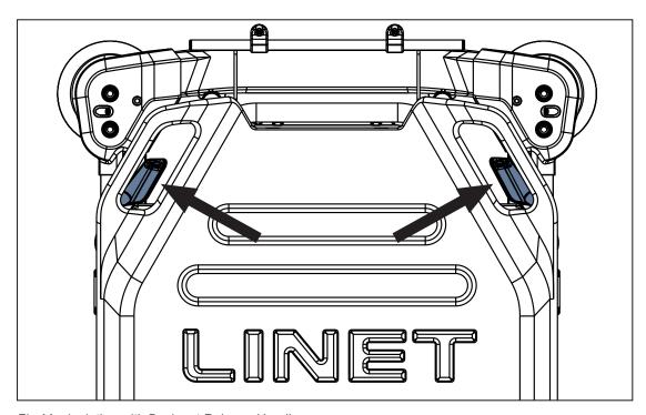
Fig. Manipulation with Backrest Release Handle
