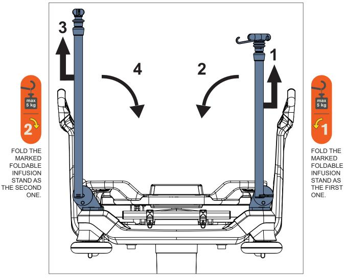
Fig. Pair of Foldable infusion stands (head end)
