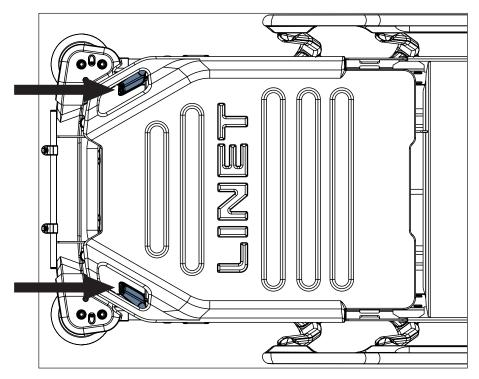
Fig. Positions of Backrest Release Handles
