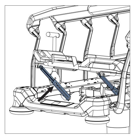
Fig. Catch in the ratchet-bar
