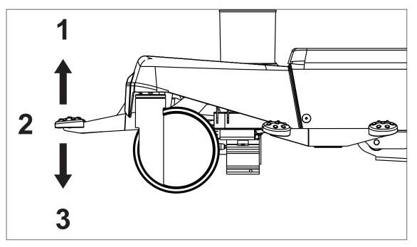
Fig. Three Pedal Positions (Green Drive Pedal)
