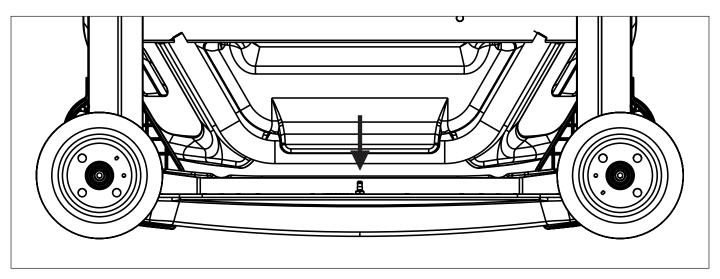
Fig. Potential equalisation - male (head end, bottom view)
