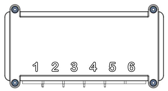
Fig. Battery Box with Cover fixed with 4 screws
