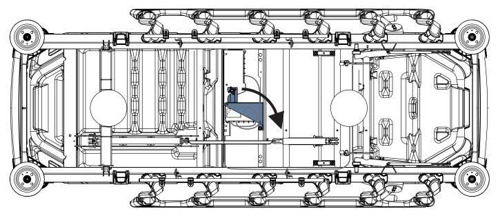
Fig. Tipping the Battery Box Holder out (bottom view)
