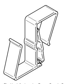
Fig. Hook for hanging Power Supply Cord
